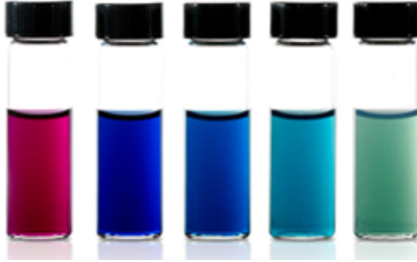
Figure 4: Color of fluid containing nano-particles can be obtained by changing the permittivity of the background fluid.
